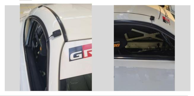
Reason: To ensure Motec dash GPS picks up the appropriate number of satellites. It has been discovered that the original fitting location shields the GPS pick up which in turn creates inconsistencies with the Motec Dash information.
