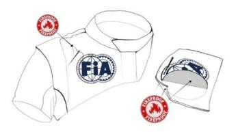
3. Addition of badges - The backing material of badges and the thread used for affixing them to the garment must be flameproof. The stitching of badges can go through all layers, provided that the thread is flameproof.
