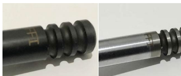
examples of FFI exhaust and inlet valve marking
