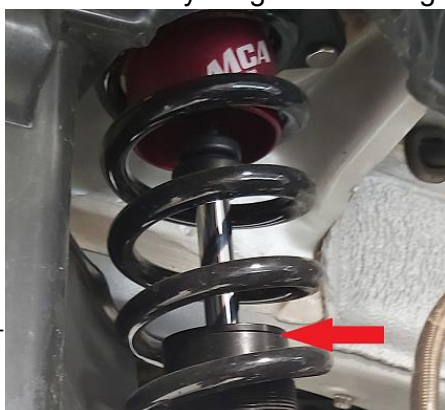
Figure 9.3.7-2 Rear Shock Absorber Body Height measuring points
