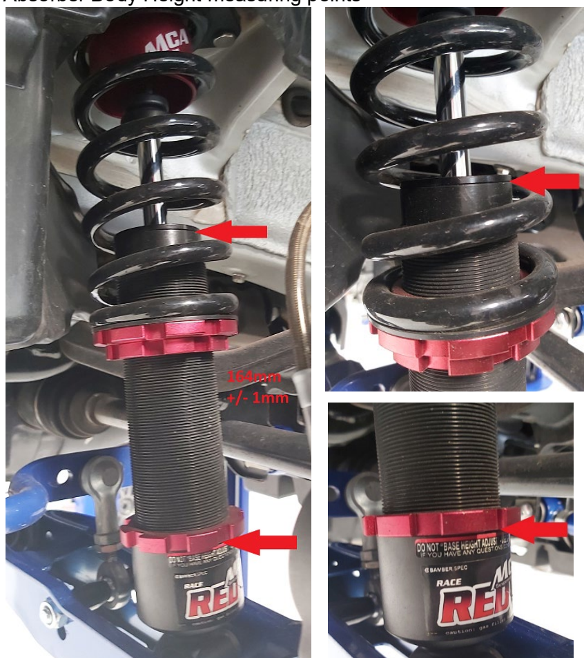
Figure 9.3.7-2 Rear Shock Absorber Body Height measuring points
