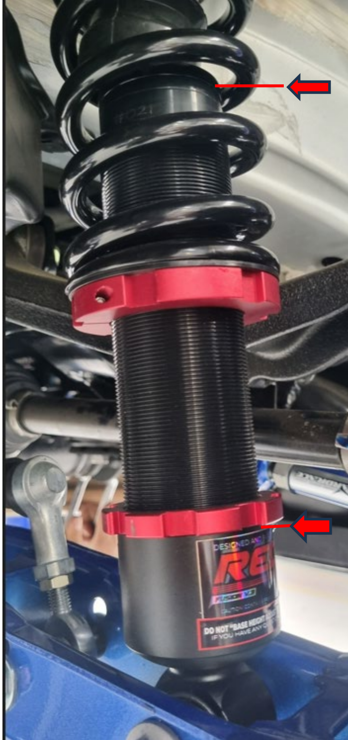
Figure 9.3.7-2 Rear Shock Absorber Body Height measuring points
