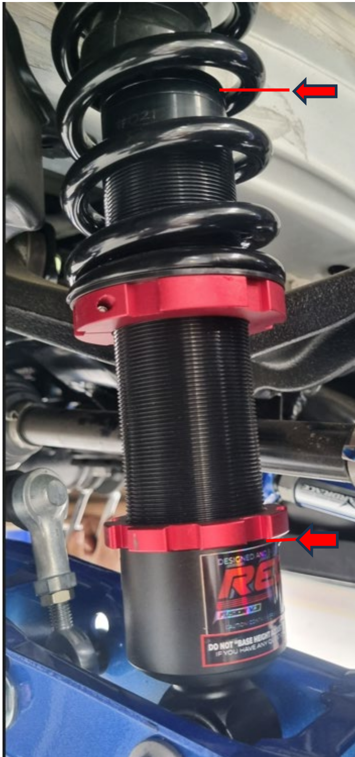
Figure 9.3.7-2 Rear Shock Absorber Body Height measuring points
