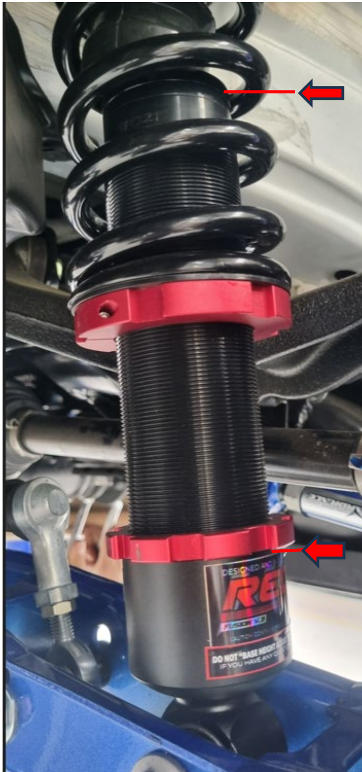
Figure 9.3.7-2 Rear Shock Absorber Body Height measuring points
