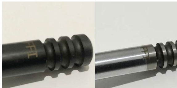
Examples of FFI Exhaust & Inlet Valve Marking
