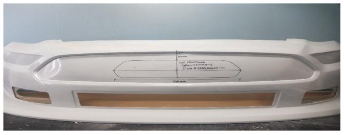
**APPENDIX 12:** Full wear strip attached to One-piece fibreglass nose assembly.
