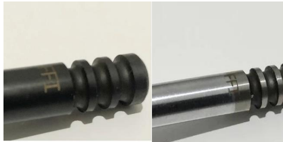
Examples of FFI Exhaust & Inlet Valve Marking
