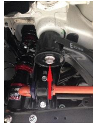
Left Rear measuring point
