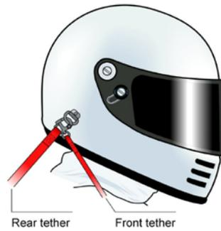
Figure 3 Identification of a Hybrid device's tethers
