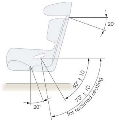
Figure 7 Side view to show recommended belt angles
